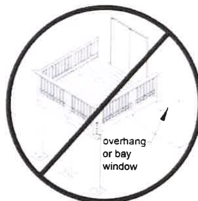
Figure 18. No Attachment to House Overhang with Ledger.
