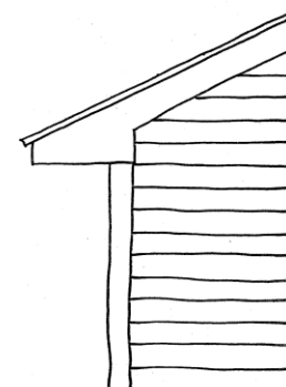
Modern boxed soffit is inappropriate for pre-1950 buildings
